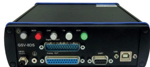
USB, fieldbus, digital IO and analog integrated
